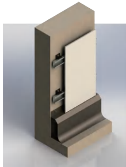
05. Waterproof footing of wall with hanging panel
